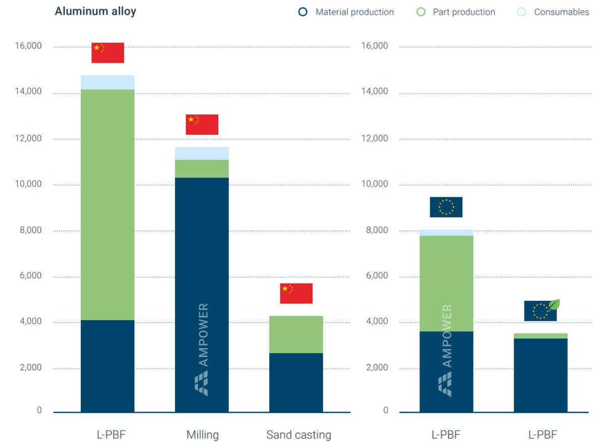
The results show the large influence the local grid has on the proportional distribution of CO<sub>2</sub> emission from material production and part manufacturing. This becomes especially evident when comparing the data for the aluminum part from the previous page, calculated with identical grid parameters.
