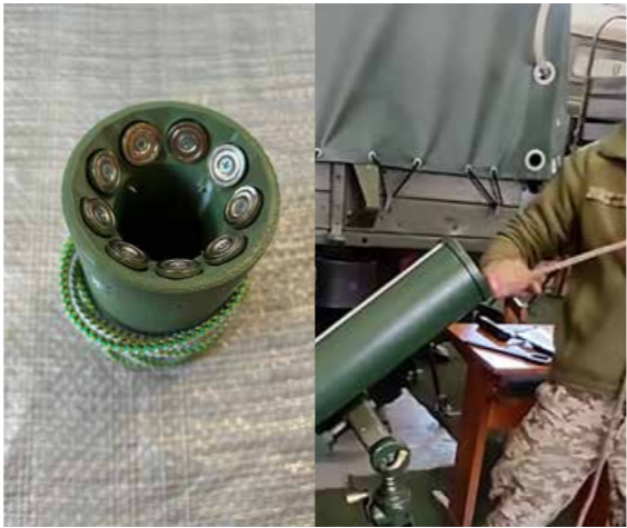
Mortar Mine Extractor — a non-lethal safety tool that enables safe removal of a stuck round from the mortar tube. Essential for frontline mortar crews.
