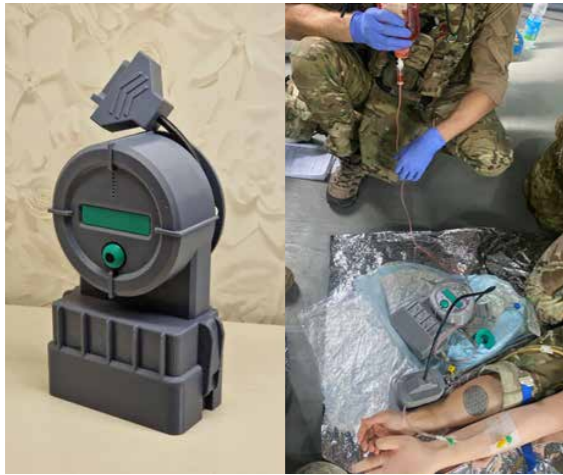
QInFlow Warrior training mock-up — full-scale 3D-printed blood-warmer. Enables setup/connection/transfusion drills, building muscle memory without risking the original; for medics, paramedics and training centers.
