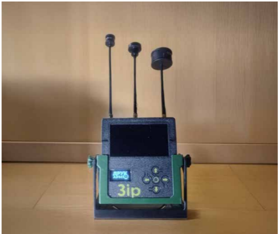
ZIR — FPV detector / video receiver: intercepts enemy FPV video; usable handheld, vehicle-mounted, or in shelters. Early warning and actionable awareness.
